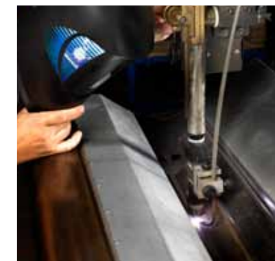
Plasma welding of stainless material in a long-seam automated device
