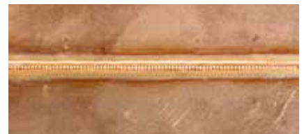
Copper – plasma-melt in 0.6 mm wall thickness
