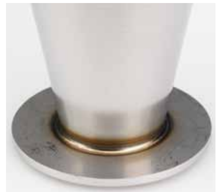
Conical pipe TIG welded onto plate. Note the thin throat thickness.
